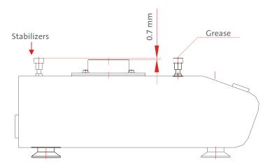
Before you attach the platform, make sure that the slide stabilizers are properly fastened, adjusted and lubricated with the included grease.
