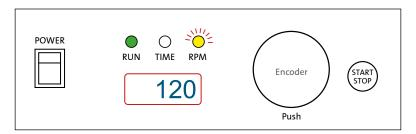
If you want to view the set value for TIME during shaking, rotate the encoder knob for ONE CLICK right (+) or left (-). Time signal light will then flash for 2 sec., and the display will show the set TIME and the light will stop flashing.
