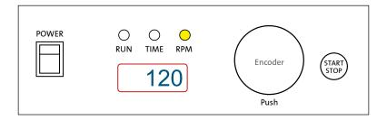
▶ Press START/STOP button to start operation. RUN and TIME signal lights. Shaker runs and counts down time from set value.
