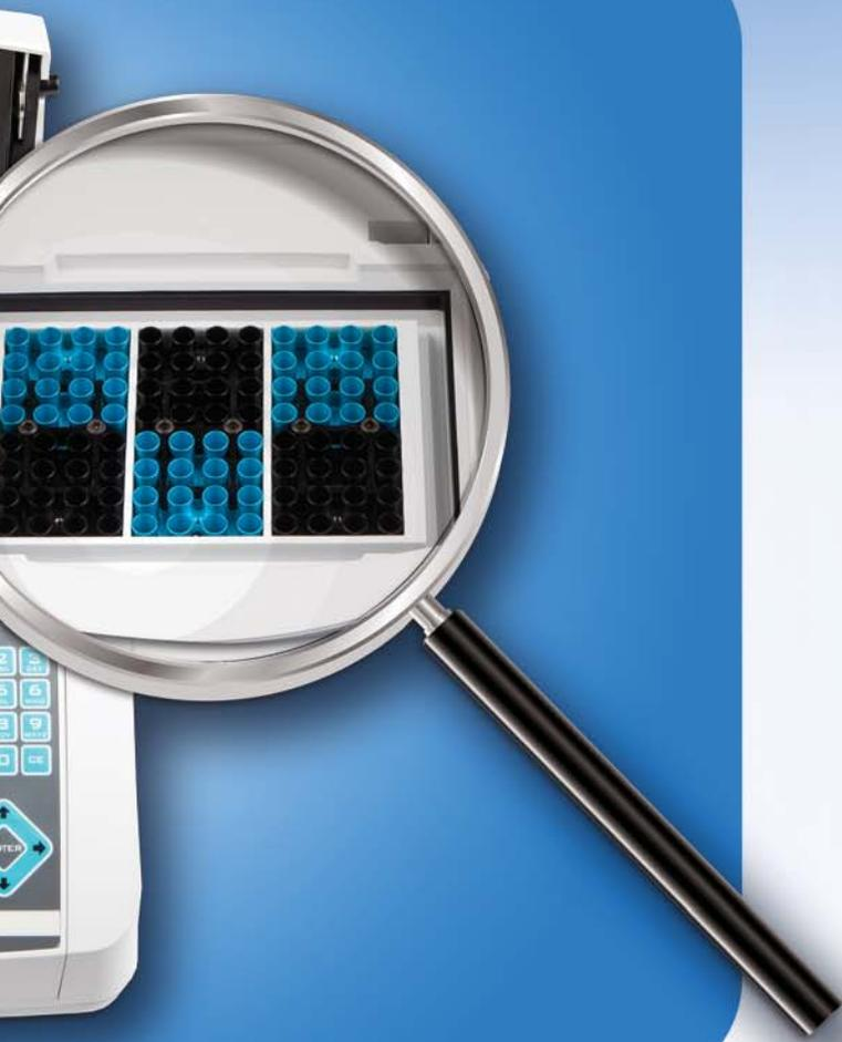
**The FlexTemp technology** provides a greater flexibility in approaching laboratory workflows. Because you can easily select annealing temperatures and because many primers work with common methods, you can run up to 16 wells of one primer at one temperature and 16 wells of another primer at another temperature during same run. The MultiGene OptiMax allows you to set 6 different temperatures. A different temperature in each of the 4 x 4 well blocks. Maximum workflow flexibility.
